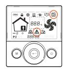
Replace the filters (supply and discharge air) with the official Vasco filter sets, which can be purchased from wholesale businesses. There is no need to reset the dirty filter warning, given that the message is displayed and triggered by the reading of the differential pressure switches in the ventilation unit. The message can be reset faster by briefly switching off the wired wall-mounted control unit.
